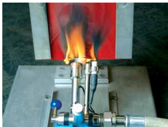
Limit of incandescence: 3 seconds after the flame is withdrawn.
