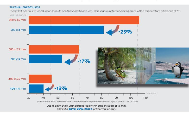
Use a 2 mm thick Standard flexible vinyl strip instead of 1,5 mm allows to save 25% more of thermal energy.
